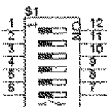
S1 DIP switch for user selection
